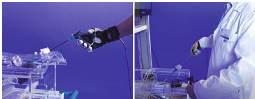
Fig. 13.1 Positions of the surgeon's hand during the recording of data using the CyberGlove ®
